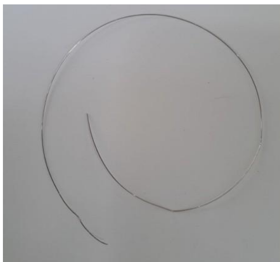
Figure 3. Stainless steelwire used to serve as electrode in artisanal electrophoresis box.
