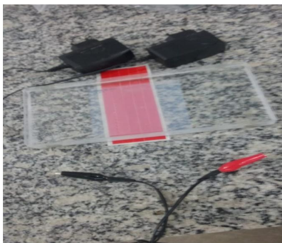
Figure 4. Opened electrophoresis recycled box showing wired clips, energy sources and
